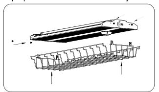
2.Insert the provided chips(4 pcs) onto the wire guard.
