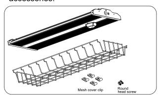
3. Fasten the chips by screws into the prepunched holes of fixture body.
