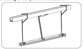
2.Connect the V-hook to back of the fixture body.
