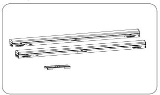
2.Install the connector to the end of the luminaires.
