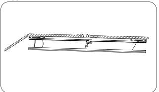
2.Fix the baffle onto the back of the fixture with screws.
