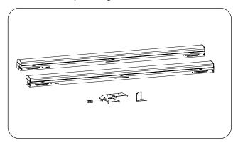
2. Secure the interconnection bracket with screws.
