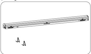
3.Attach the V-hooks to the fixture body to hang the luminaire.
