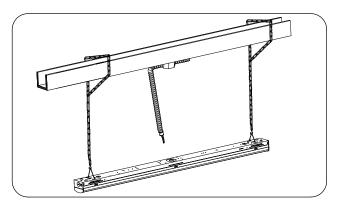
5. Reattatch the luminous part to the housing to complete the installation.
