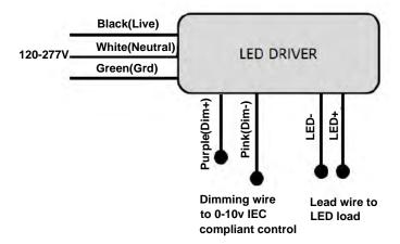
Note: The CCT-adjustable function integrated Driver will have one more "LED-" output wire.
