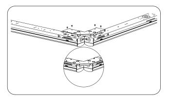
3. Secure the interconnection endcover with screws.
