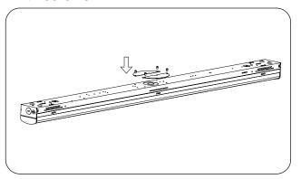
4.Pull AC wires and dimming wires through the outlet hole, then fix the luminaire to the ceiling with anchors and screws(not included).
