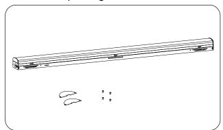
3. Open the luminous part down by pressing the area between the narrow strip hole and snap-lock.
