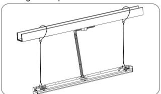
2. Attach V-hooks to the cable.
