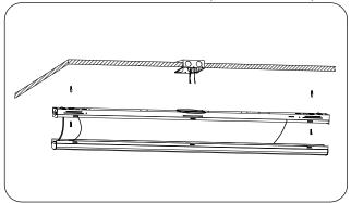
6.Assemble the luminous part upwards. The installation is completed.
