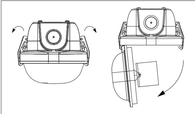
2. Connect an appropriate length of power cord to driver as shown in below figure<sup>[1]</sup>. (the flexible cord supplied by others)
