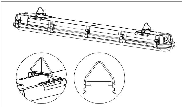
4. Hang the fixture by attaching the V-hooks to chains. Make wiring connection to Power supply accord to local laws and regulations.
