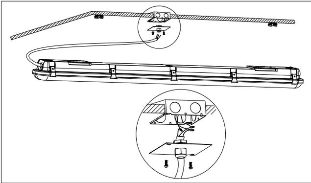
6. Press fixture housing to the clips until both sides of the housing recesses are secured.
