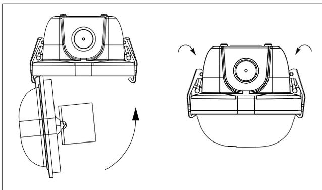
4. Locate and drill holes, then install clips to the ceiling surface using hardware found in hardware kit.
