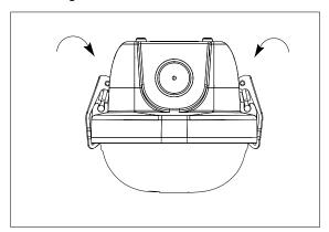
2.Press fixture housing to the clips until both sides of the housing recesses are secured.
